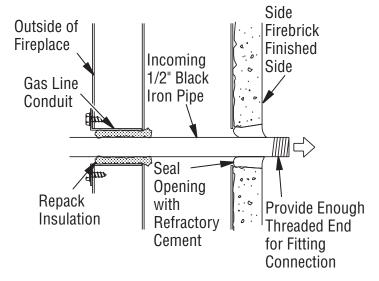
Figure 19 - Gas Line Installation
