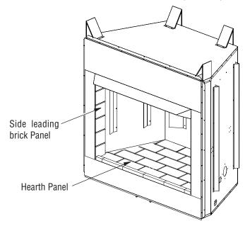
Figure 13 - Installing Hearth and Leading Brick panels
