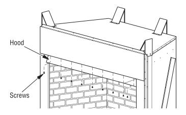
Figure 16 - Installing Hood
