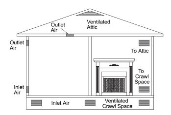
Figure 5 - Ventilation Air from Outdoors
