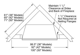
Figure 9 - Corner Installation
