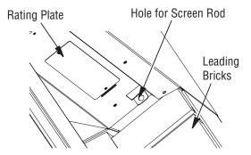
Figure 17 - Installing Fireplace Screen
