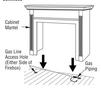
Figure 11 - Installing Cabinet Mantel (Mantel May Vary From Illustration)
