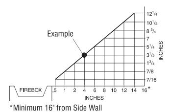
Figure 6 - Minimum Clearance for Combustible to Wall
