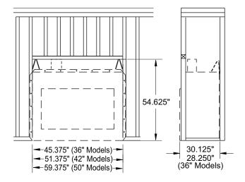
Figure 8 - Framing Dimensions
