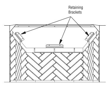
Figure 15 - Installing Side and Rear Walls
