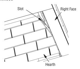
Figure 14 - Slots for Firebrick Walls
