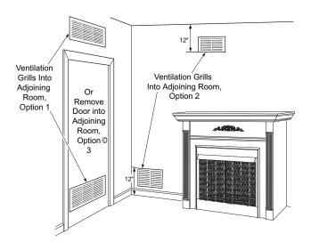
Figure 4 - Ventilation Air from Inside Building
